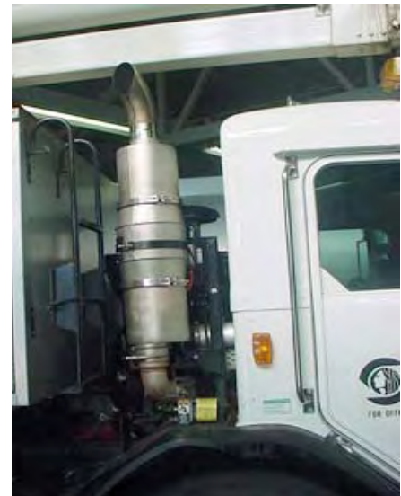
Catalyst and filters shown installed on truck exhaust pipe clean truck emissions.
